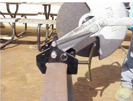
**Rail Side Cutting with Operator's Position
