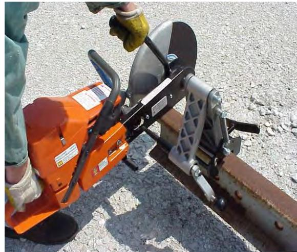
**Mounting the Ultra Kut III Saw**
