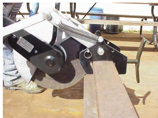
**Rail Side Cutting with Operator's Position
